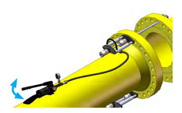
11. Continue priming the Hand Pump untill the actuators have reached full stroke 100mm (4").
