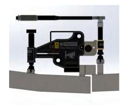
Tighten the screw bolt in a clockwise direction until the flanges come into alignment.
